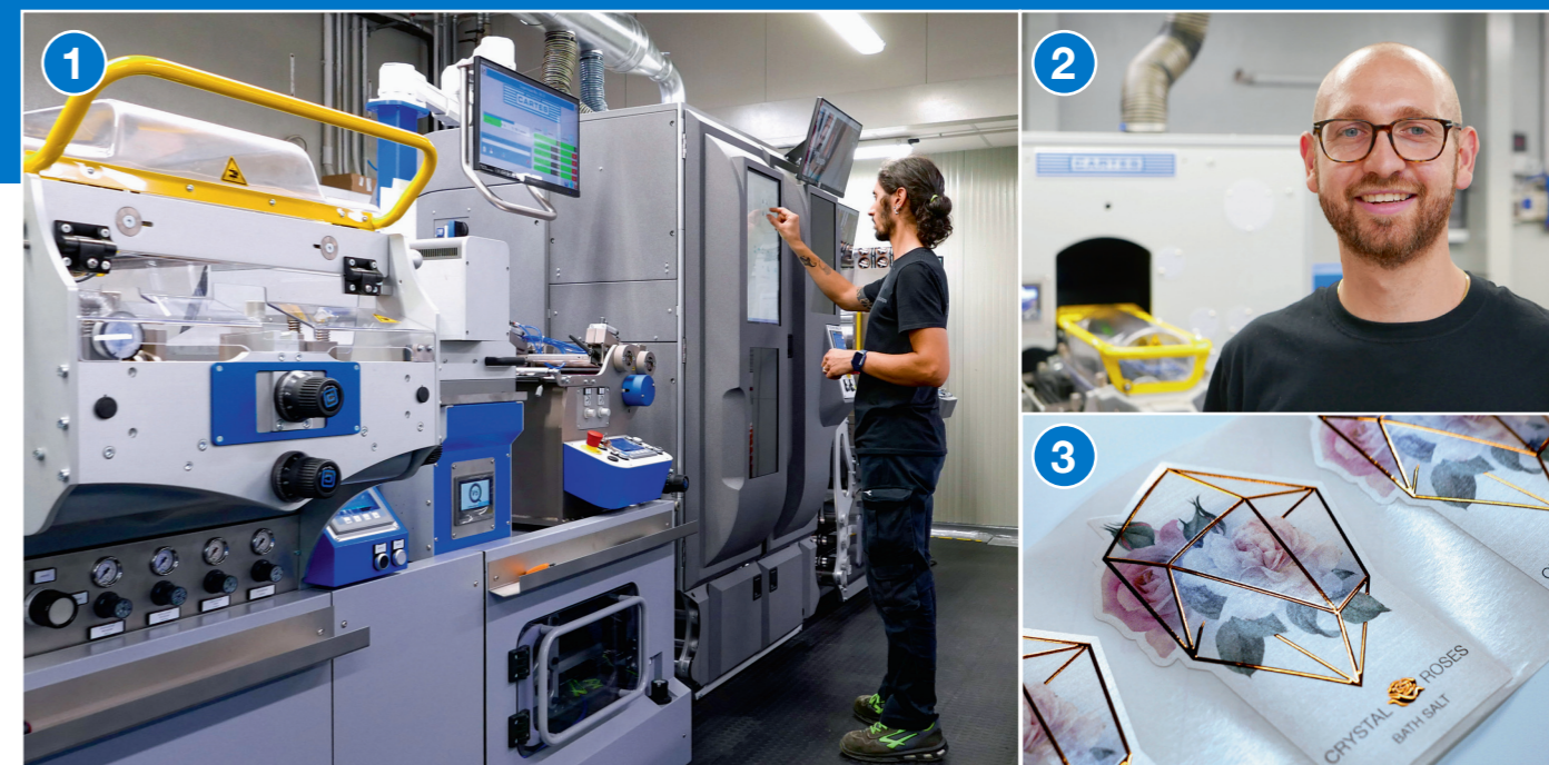
1) CARTES machine set by semi-rotary flexo, flat bed silk screen & hot stamping, JDS Digital embellishment and semi-rotary die-cutting 2) Mr. Daniele Lelli ( Multistampa Co-Owner ) 3) Label embellished with CARTES JDS
